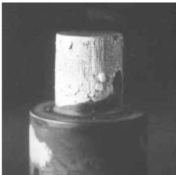
Soldering damage on a core pin.
