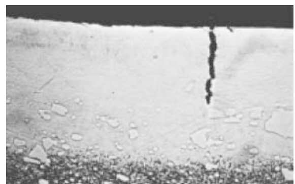
Fig. 6e. Graphite electrode. t_1 = 500 \mu\text{s} . Magnification 500 X
