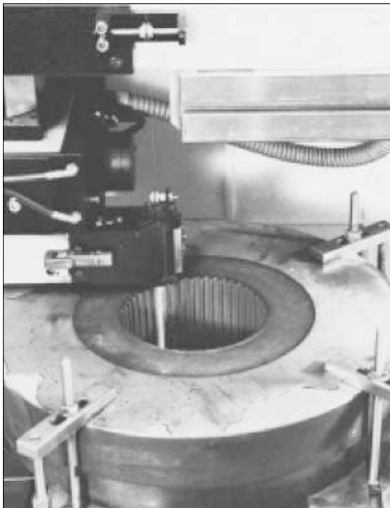
Fig. 11. Wire erosion of a hardened and tempered tool steel blanking die.
