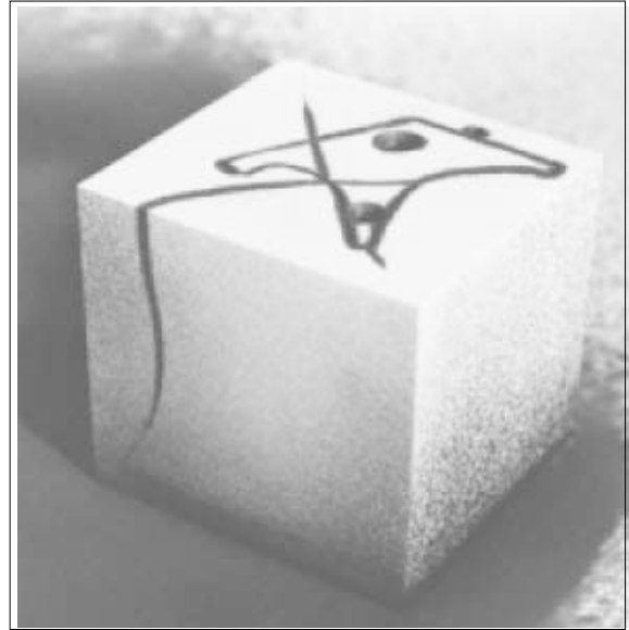
Fig. 12. This block of D2 steel, approx. 50 x 50 x 50 mm (2" x 2" x 2"), cracked during the wire EDM operation.
