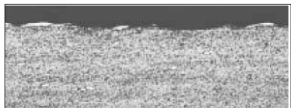
Fig. 5. Fine-machined RIGOR. Pulse duration 10 μ sec.
