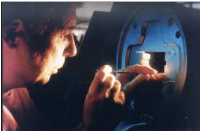
Manufacturing of dies (SAPA, Sweden).
