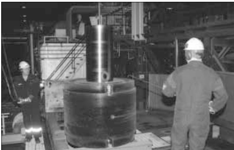
Shrinking of liner.
