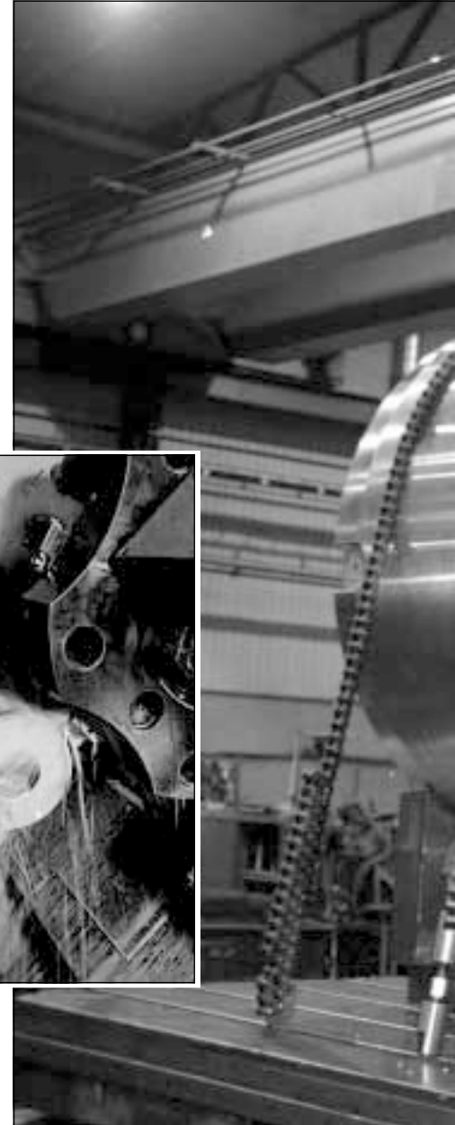
CNC-turning of dummy block in heat treated condition.
