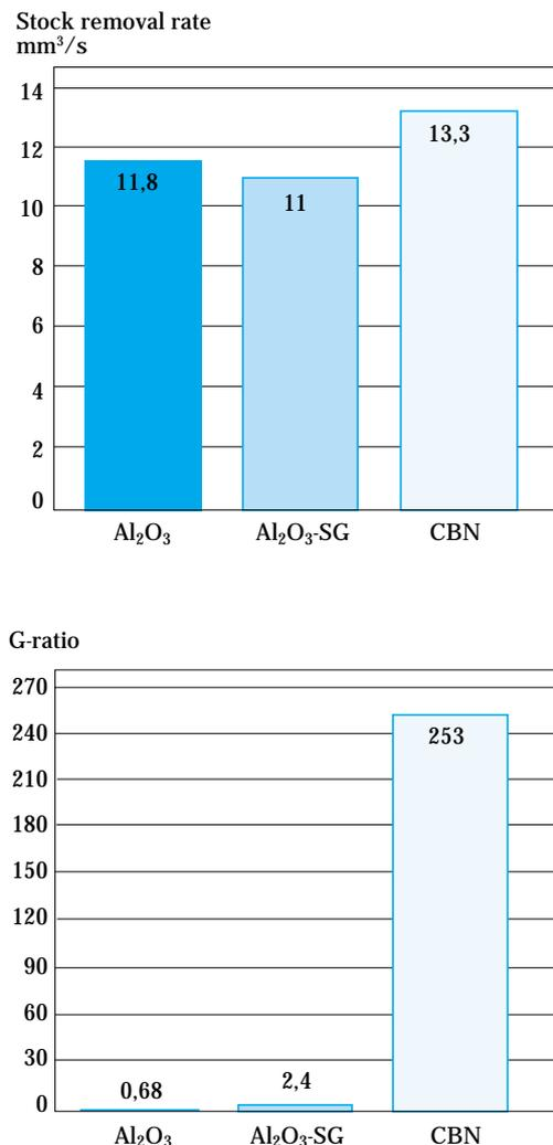
Figure 10. Surface grinding of *VANADIS 10* with various grinding wheels. (Grinding wheel width: Al<sub>2</sub>O<sub>3</sub> 40 mm, CBN 20 mm.)
