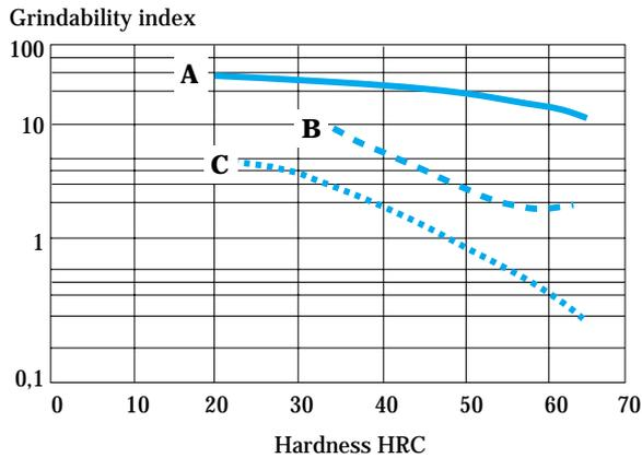
Figure 6. The effect of hardness on grindability for:
