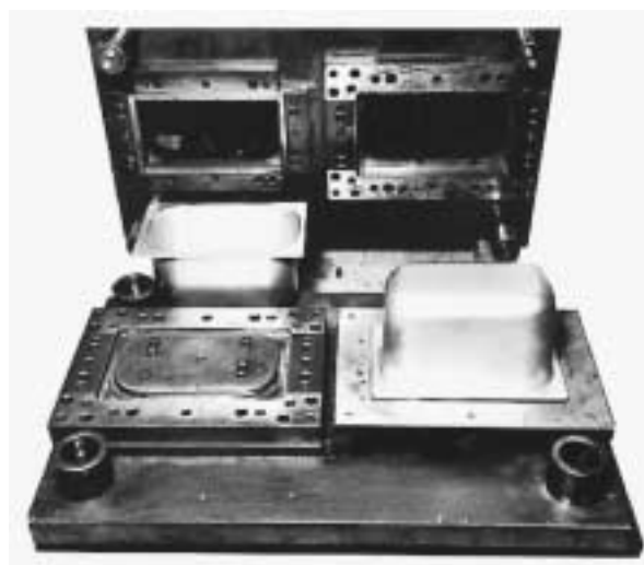
Clipping and edging tool in ARNE tool steel to clip and form edge of 0,914 mm (0,036") thick stainless steel container approx. 254 x 152 x 203 mm (10" x 6" x 8").
